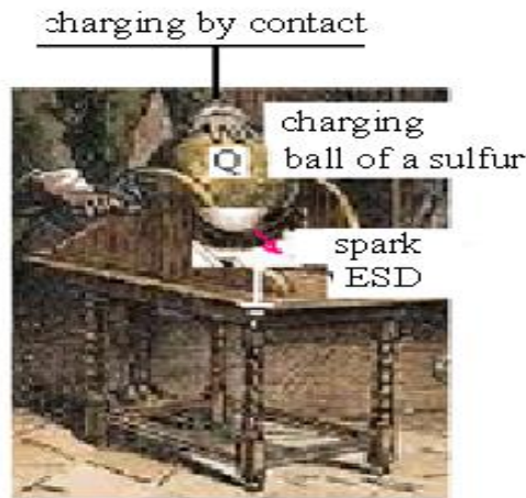
Figure 4: Prototype electrostatic machine Otto von Guericke.
